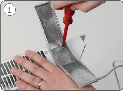
Fit the aluminium feet into position using the supplied screws.
