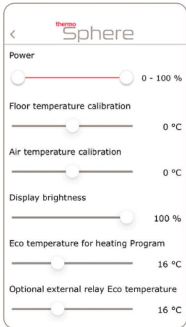
**Power:** Use to limit the surface temperature of electric panel heaters.
