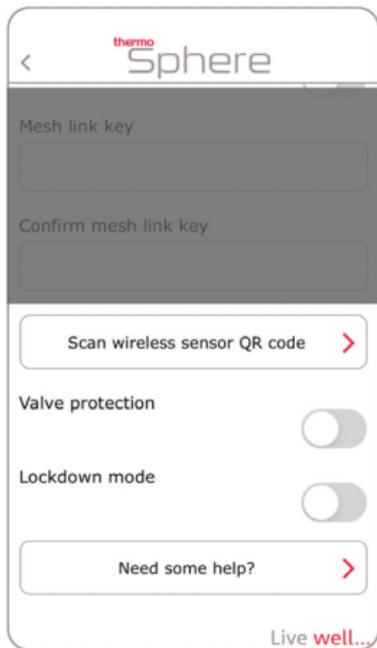
**Wireless sensor:** You can connect a compatible wireless temperature and humidity sensor (required for Snow melting).
