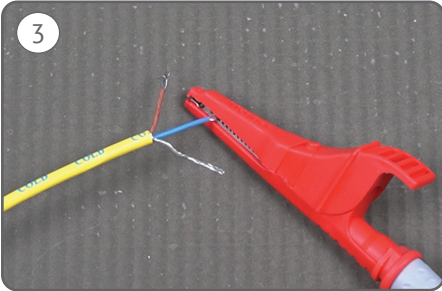
3 Connect one of the clips to the Neutral (Blue) wire.
