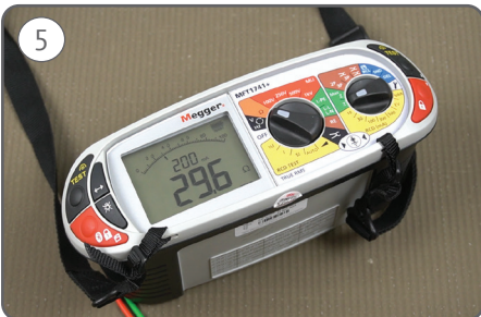
5 Check the meter reading is within -5 to +10% of the manufacturer's value on the labels.
