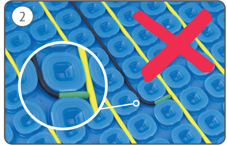
Note: Don't position your sensor near or under heating cable.
