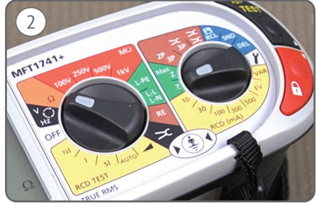
2 Turn your test meter on and set to Ohms ( \Omega ).
