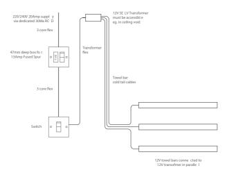
ThermoSphere Towel Bars are 12V SELV and can be installed safely anywhere in a bathroom. All electrical circuits in bathrooms must be protected by a suitably rated RCD.
