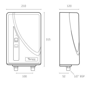
The instant heating Micro Electric Boiler for heating and hot water applications. Save space, installation time and running costs compared with other electric water heaters.
